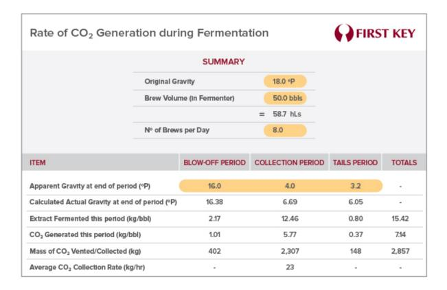
Note: Typically 1.5 vols/vol of  $CO_2$  per volume of beer remains dissolved in the beer out of fermenting. This equates to 0.327 kg  $CO_2$  / bbl. This quantity dissolves during the Blow-Off period so that all the  $CO_2$  generated during the Collection Period is available for collection.
